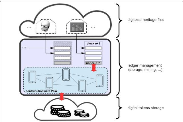
**Fig. 4** The ledger layer and the consensus layer of a novel cultural heritage IT architecture (block n + 1 is being mined, while the previous block has already been mined and already provides integrity)
