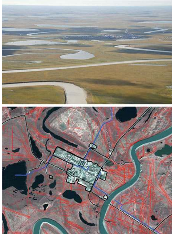
Fig. 9.3 (top) Landscape and main developed area in the Bovanenkovo gas field. Reproduced by permission of D.A. Walker. (bottom) Quickbird image of the main developed area. Colored lines were digitized for GIS analysis and show construction pads for buildings and storage and roads (black), pipelines (blue), and off-road vehicle trails (red). Reproduced by permission of Timo Kumpula
