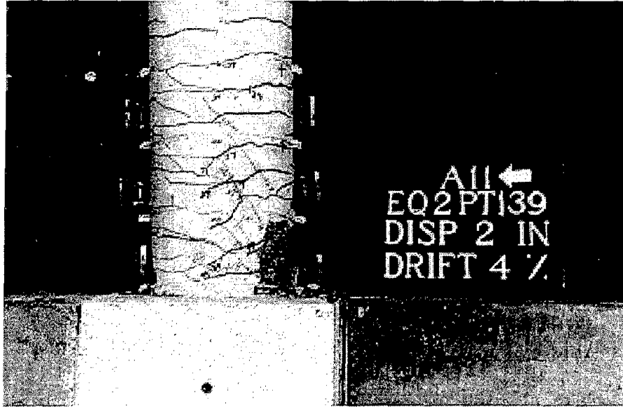
FIGURE 5-20 Specimen A11 at Half-Cycle # 139
