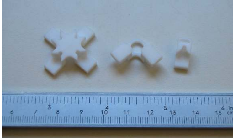
Figure 6. The three types of PTFE holders used for the tower construction.
