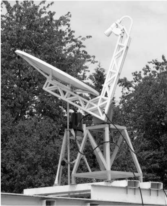
Figure 1: Picture of the CURIE offset antenna at the top a shelter at the SIRTA site (Ecole Polytechnique Palaiseau, France). The antenna is fixed to a positioning system at the left of the picture.
