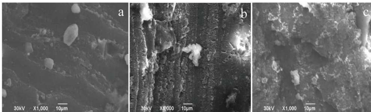
Figure 6: SEM images of GTR/NR: (a) 30/70, (b) 50/50, (c) 70/30 blends.
