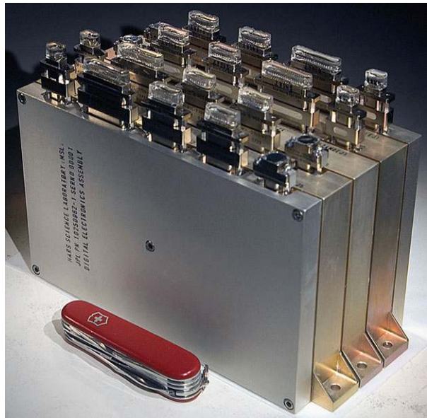
Fig. 9 Digital Electronics Assembly (DEA) package for Curiosity's MAHLI, two Mastcams, and MARDI. Each instrument DEA is a separate entity (they do not communicate with each other); they were packaged together to reduce volume and mass. The pocket knife is 88.9 mm long
