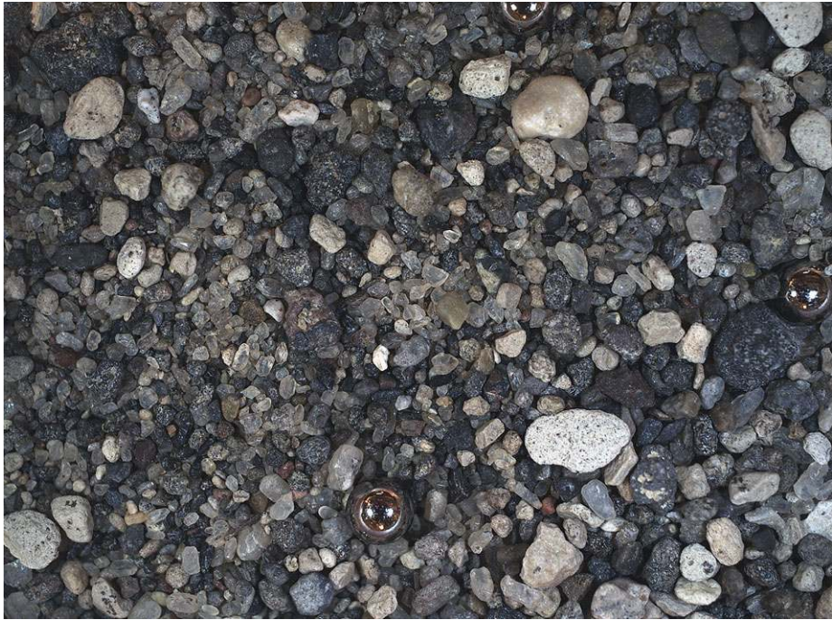
Fig. 17 Example image of regolith fines acquired by the testbed-MAHLI on 18 May 2010. Three 2 mm-diameter steel balls indicate scale. This view covers an area about 2.5 cm by 1.8 cm. The sample is a volcaniclastic eolian dune sand collected in eastern Christmas Lake Valley, Oregon. The sand includes basalt fragments, pumice, and plagioclase crystals
