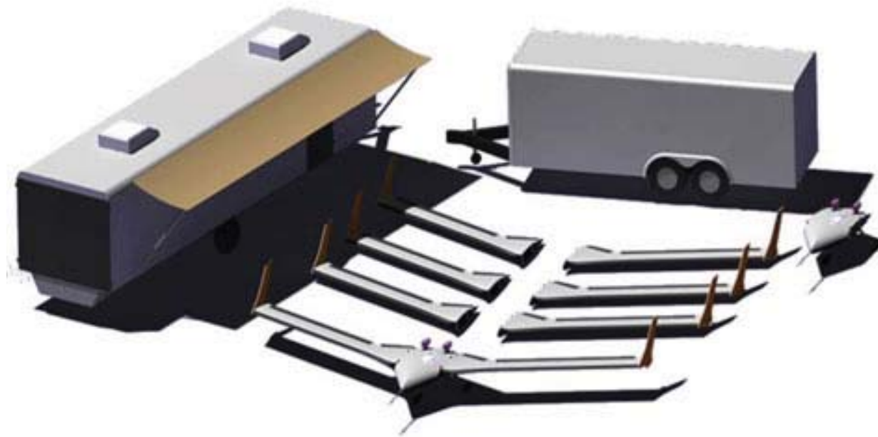
Figure 1. The X-56 aircraft system consists of two center-bodies, four wing sets, a ground control station, and a storage trailer.
