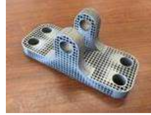
(b) Variable-density periodic lattice infill [20]
