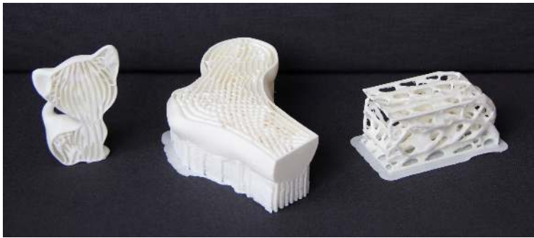
(c) High-resolution voxel-based porous infill [26]
