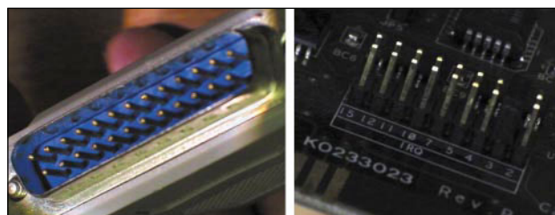
Figure 1 Gold plated computer D plug and connector pins on a computer PCB
