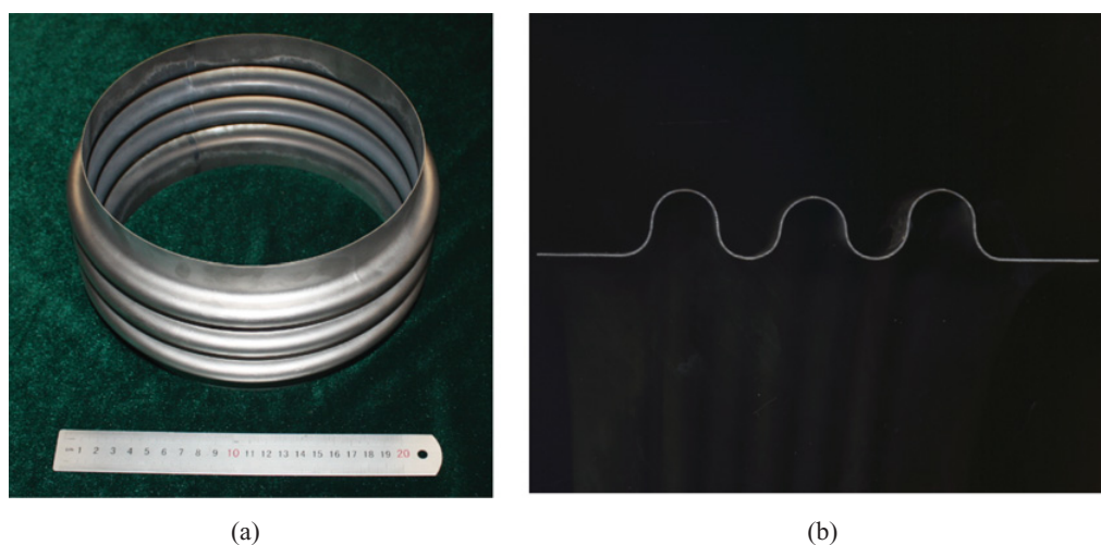
Figure 7. Large-size bellows of titanium alloy: (a) integral drawing, (b) sectional drawing.
