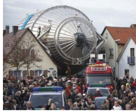
FIGURE 20: Photograph of the spectrometer transport during the final careful maneuvering through the nearby village of Leopoldshafen in November 2006. Due to its size, it could not be transported to Karlsruhe on motorways, but had to travel nearly 9000 km through the Danube River, the Black Sea, the Mediterranean Sea, the Atlantic Ocean, the North Sea, and the River Rhine [139].
