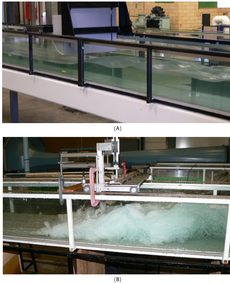
Fig. 1. Photographs of hydraulic jump flows. (A) Undular hydraulic jump – flow conditions: Fr_1 = 1.35 , d_1 = 0.090 m, Re = 1.1 \times 10^5 – flow from left to right. (B) Hydraulic jump with roller – flow conditions: Fr_1 = 7.0 , d_1 = 0.024 m, Re = 8.1 \times 10^4 – flow from left to right.
