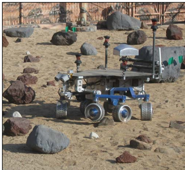
Figure 6 FIDO Rover in Mars Yard at JPL, October 2004. OASIS has identified an interesting rock for the rover to investigate (see white rock directly in front of FIDO). The green flags show the human observers where the regularly-scheduled science events should occur.
