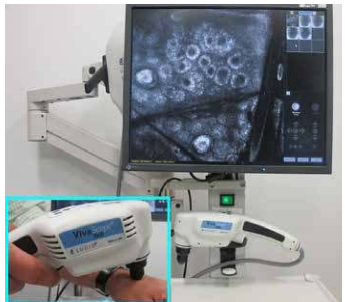
■ FIGURE 2. Vivascope Reflectance Confocal Microscope System (Lucid, Inc, Rochester, NY). Inset shows the handheld Vivascope 3000.
