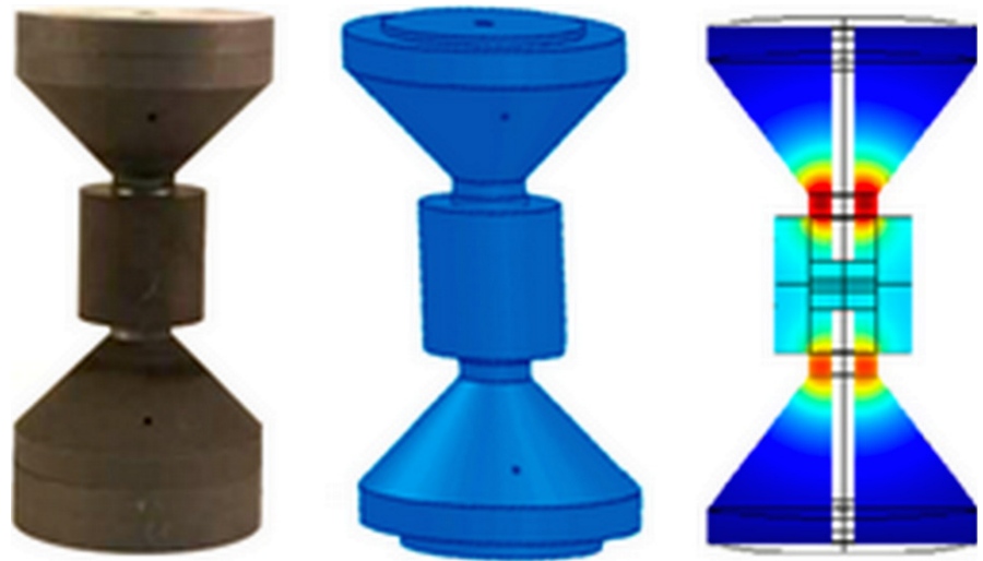
FIGURE 15 SPS die-punch set-up: photo (left); CAD model (middle); and 3D FE modeling of SPS processing (right). FE modeling shows nonuniformity of temperature distribution in SPS tooling 269
