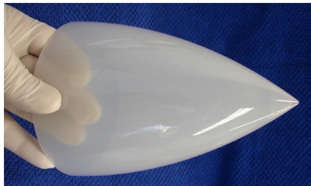
FIGURE A3 CeraLumina ™ alumina dome (Courtesy of CeraNova)
