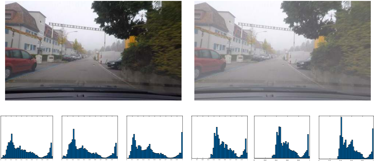
Fig. 4 Top row, left to right: example input image from Foggy Zurich and synthesized output image with our fog densification. Bottom row, left to right: R, G, and B histogram of the input image, R, G, and B histogram of the output image
