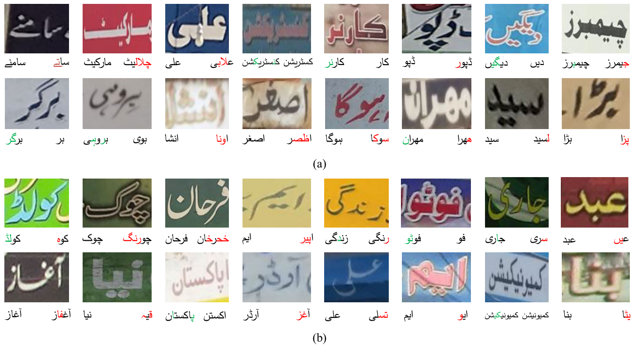
FIGURE 14. Qualitative results of incorrectly recognised cropped Urdu scene text using the (a) proposed I model and (b) proposed II model. Green text at the bottom left of a word image indicates the missing characters in the predicted text, while red text at the bottom right indicates the incorrectly recognised characters.
