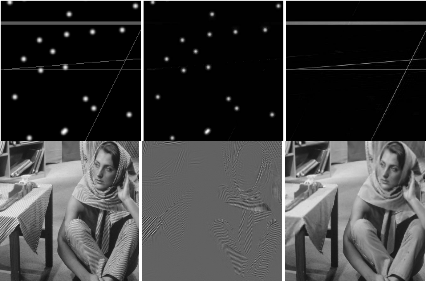
Figure 19: First row, from left to right: original image containing lines and Gaussians, separated Gaussian component (wavelets), separated line component (ridgelets). Second row, from left to right: original Barbara image, reconstructed local discrete cosine transform part (texture), and piecewise smooth part (curvelets).
