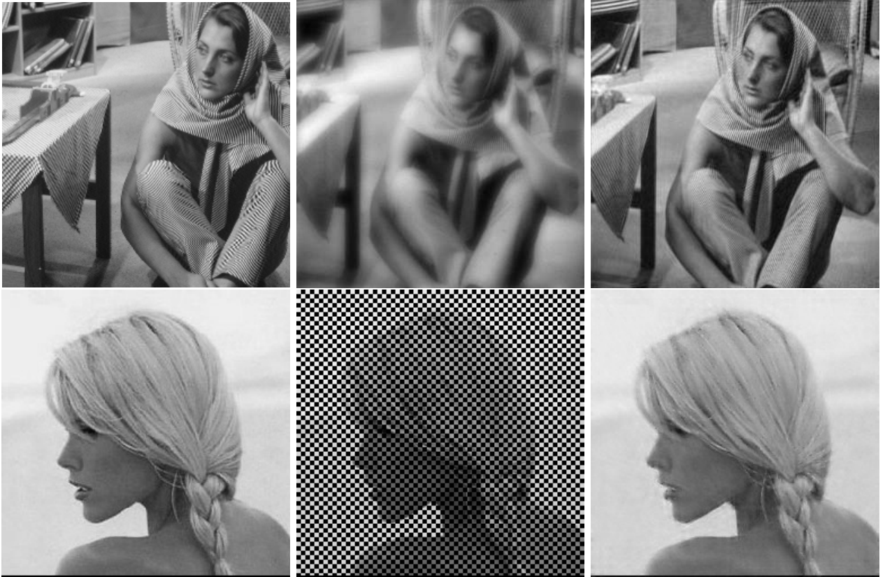
Figure 17: Illustration of the use of curvelets (DCTG2 transform) when solving two typical linear inverse problems: deconvolution (first row), and inpainting (second row). First row: deconvolution of Barbara image, original (left), blurred and noisy (middle), restored (right). Second row: inpainting of Claudia image, original (left), masked image (middle), inpainted (right).
