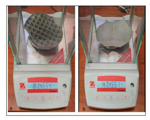
Figure 9. Weighing scale reading of cranial implant with (a) support and (b) without supports.
