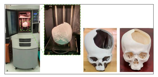
**Figure 5.** (a) Stratasys Dimension Elite FDM machine used for the fabrication of defective skull. (b) The defective skull with supports and (c) after support removal.
