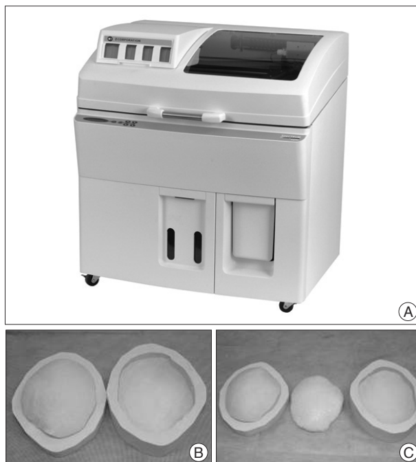
Fig. 4. By using three-dimensional printers (Spectrum Z510 3D printer from Z Corp.) (A), molds are prefabricated through powder depositional modeling processes (B). Intraoperatively, the polymethyl methacrylate implant is made by the prefabricated mold and casting (C).
