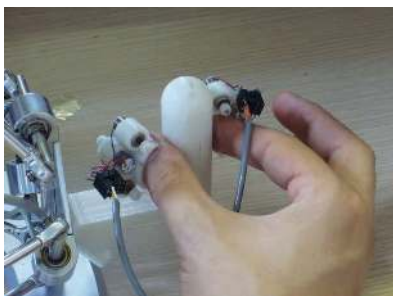
Fig. 3. The haptic handle grabbed by the operator using two fingers and two wearable cutaneous devices.
