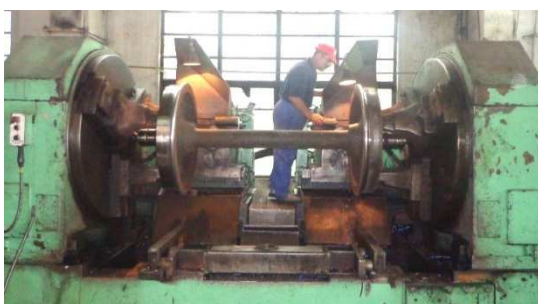
Fig. 2. Front view of the RAFAMET UBC 150 lathe
