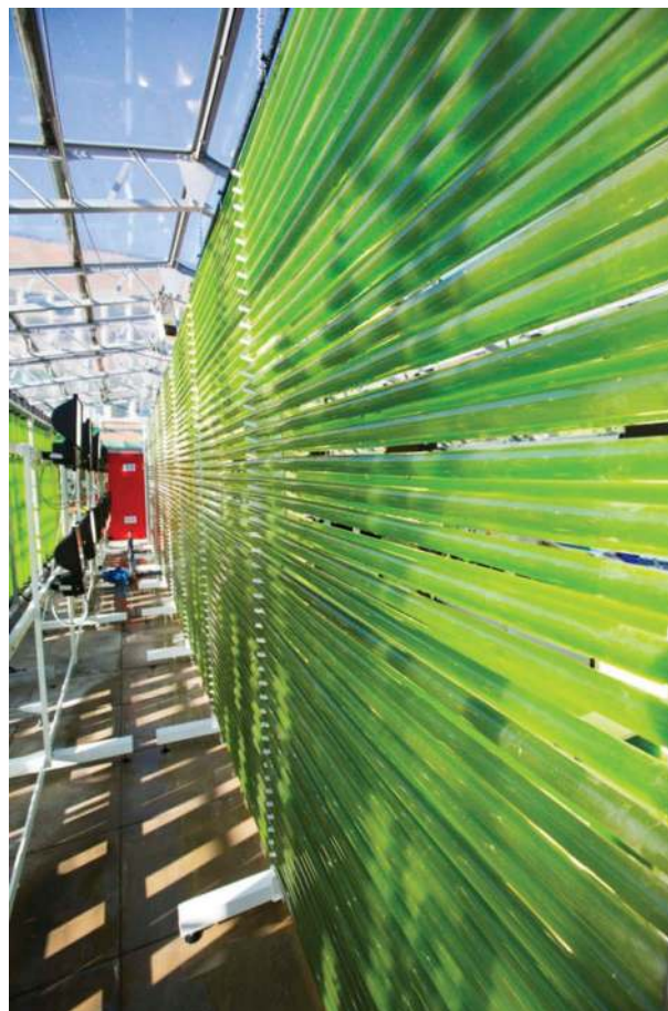
Fig. 6. A bioence photobioreactor used for the cultivation of photosynthetic microorganisms at the Centre for Sustainable Aquatic Research, Swansea University.
