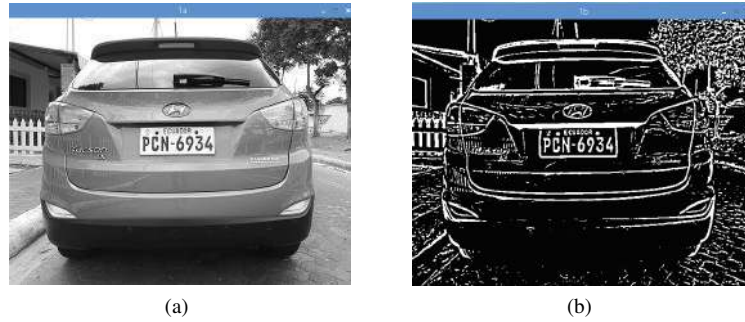
Figure 4. License plate image, (a) in gray-scale (b) in binary
