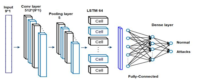
Figure 6. CNN–LSTM model for detecting attacks.
