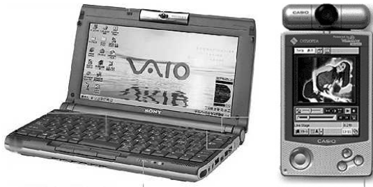
Figure 2: Examples of camera-equipped mobile devices (left: Sony VAIO notebook PC. right: CASIO Palm-size PC).
