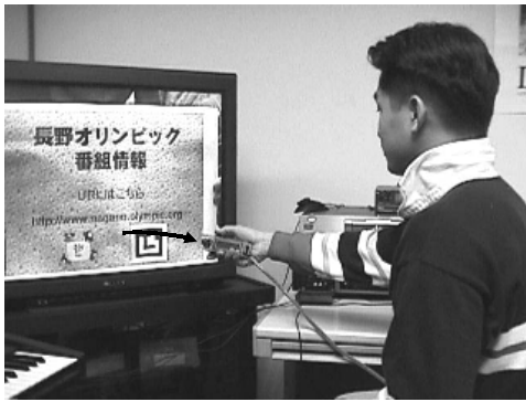
Figure 13: Retrieving ID information from a TV screen. After this operation, the user can drop the ID on a web browser and open the corresponding web page.
