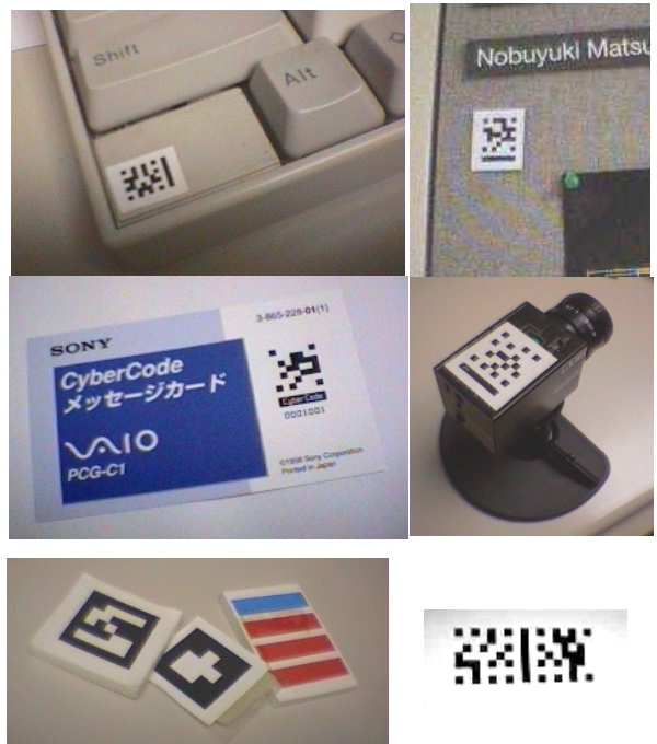
Figure 1: Examples of CyberCode visual tags (top: tags used in several contexts. bottom left: earlier prototypes. bottom right: a concatenated type for more "bits").
