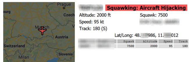
Fig. 7. Fake distress squawk code in the Dump1090 net.
