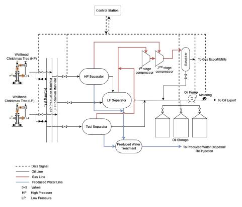
Figure 4: Upstream oil and gas production process
