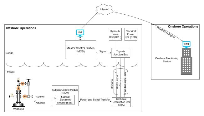
Figure 7: Example of an offshore subsea production monitoring system
