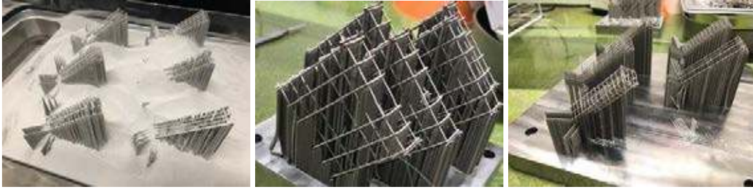
Figure 5. Left: 3D printer Jobbox. Center: Reinforcement cage after the printing process. Right: Footing reinforcement after the printing process.
