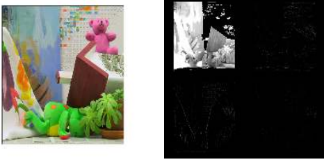
Fig. 2. (a) Cyclopean image for the "teddy" pair and (b) its color wavelet transform
