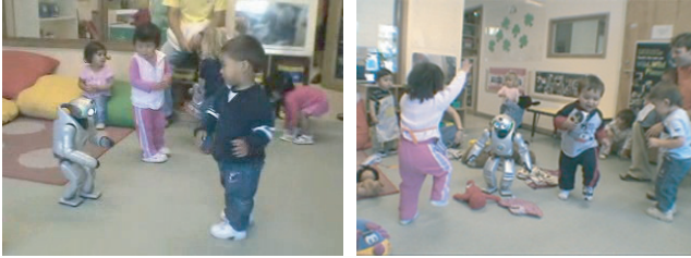
Figure 4: (Left) Canned dance: QRIO is dancing in the playback mode where there is no interactivity with the outside. (Right) Interactive dance: QRIO is mimicking the external motion dynamics.
