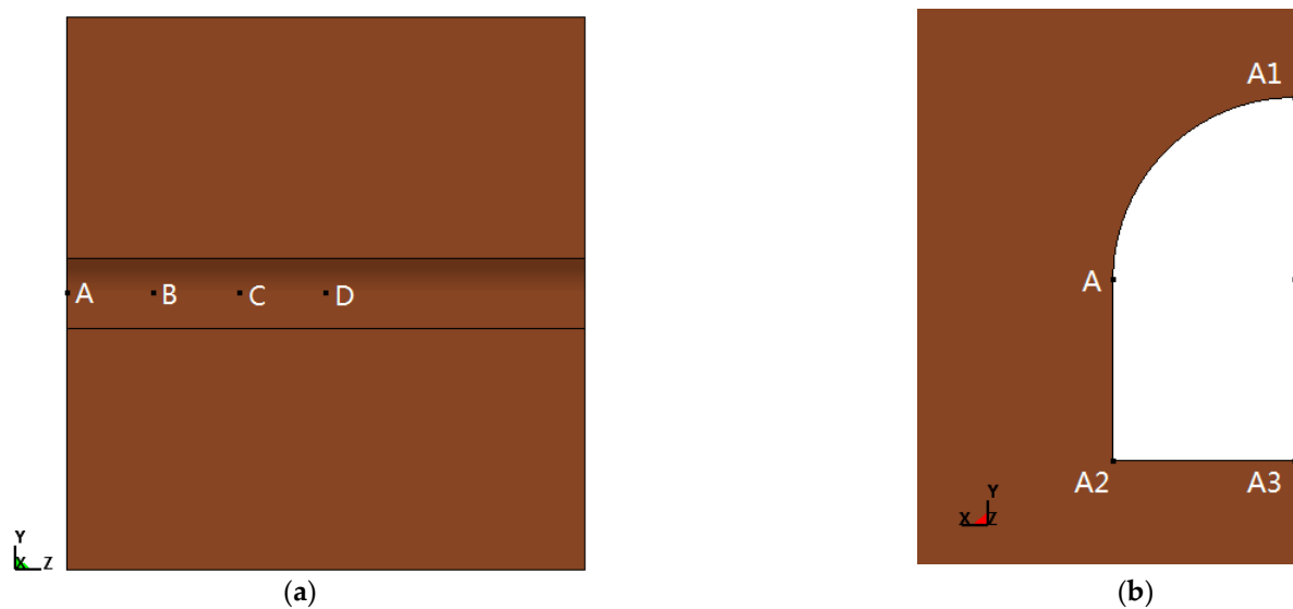
Figure 4. Positions of measuring points. (a) Wall measuring point of roadway axis and (b) Wall measuring point of roadway section.
