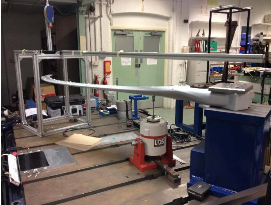
Figure 1: The experimental configuration of the WT blade, showing the geometric boundary conditions.
