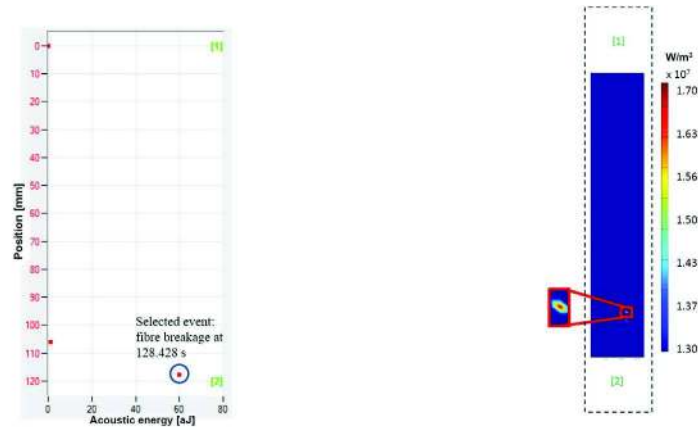
(a) acoustic events energy during interval t = 128.428 \pm 0.5 s (b) heat source field at t = 128.407 s
