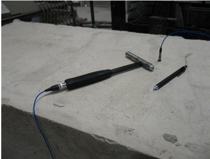
Figure 18: Impact-echo laboratory testing impact hammer and accelerometer
