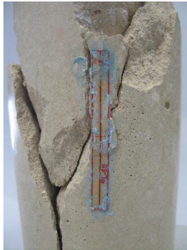
Figure 22: PL-60-11 strain gauge attached to a cylinder
