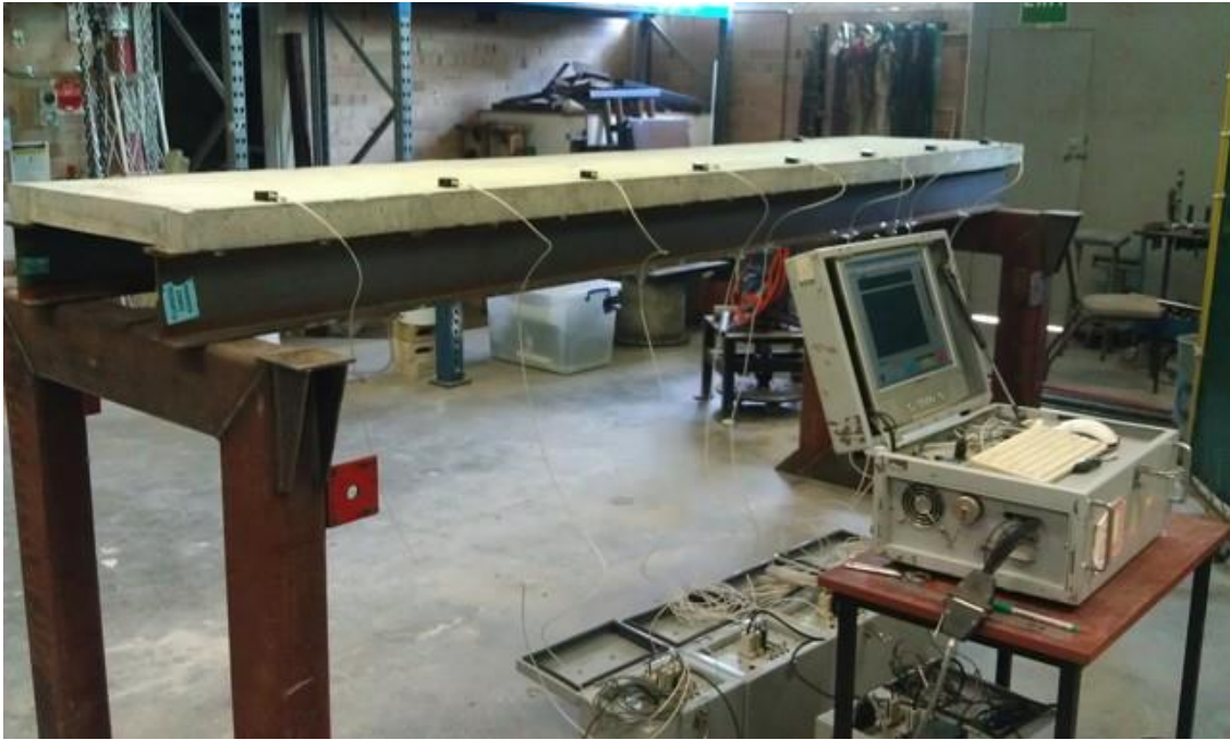
Figure 11 - Experimental test setup of the slab-on-girder structure
