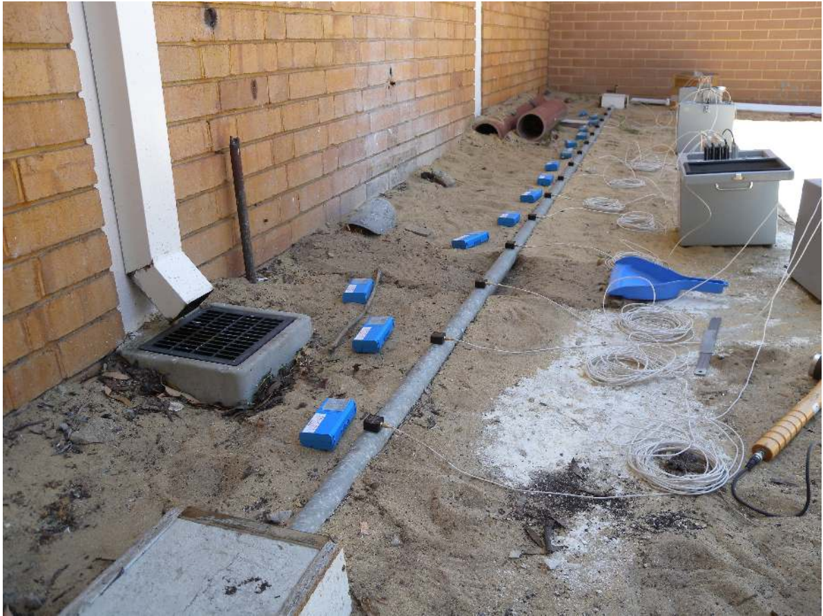
Figure 2. Pipeline test model
