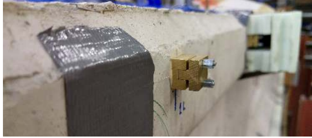
Figure 15: A typical connection of the clamping system.
