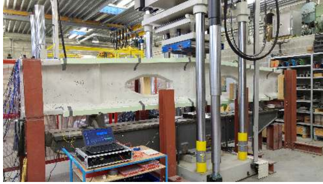
Figure 1: The experimental setup of the modal test and the PDT.
