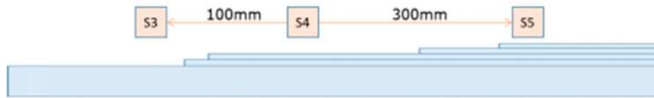
Figure 7. Schematic of plydrop specimen with the linear AE sensor array (dynamic test).
