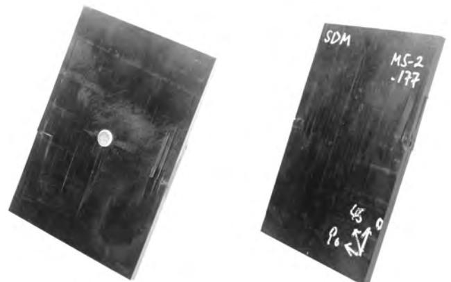
Fig. 25 70 kA lightning strike specimen (left) and 25 ft · lb (33.89 J) impact specimen (right) following residual strength CAI testing.
