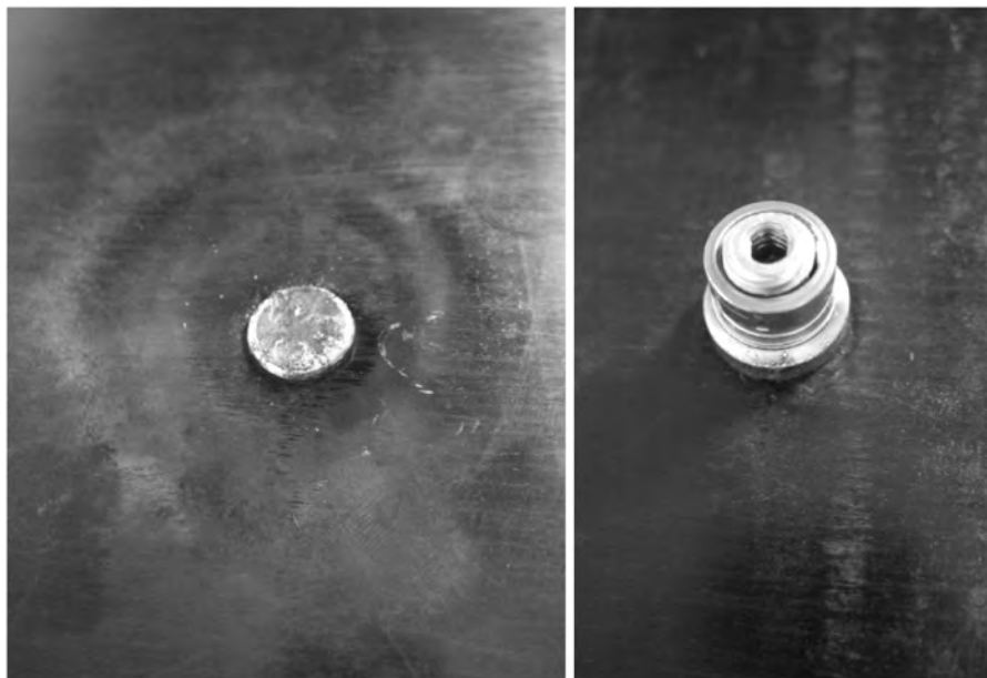
Fig. 6 Close-up of top and bottom surfaces of a filled-hole specimen subjected to a 50 kA strike.
