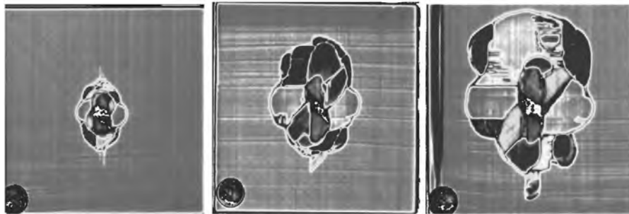
Fig. 9 Ultrasonic C-scan of the postimpact specimens at 5 ft · lb (6.78 J), 15 ft · lb (20.34 J), and 25 ft · lb (33.89 J).
