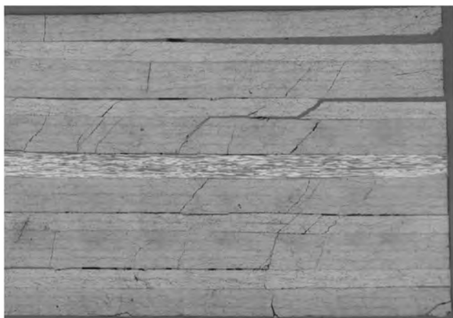
Fig. 15 Detail of the specimen impacted at 15 ft · lb (20.34 J) perpendicular to the 0 deg fibers and underneath the point of impact.
