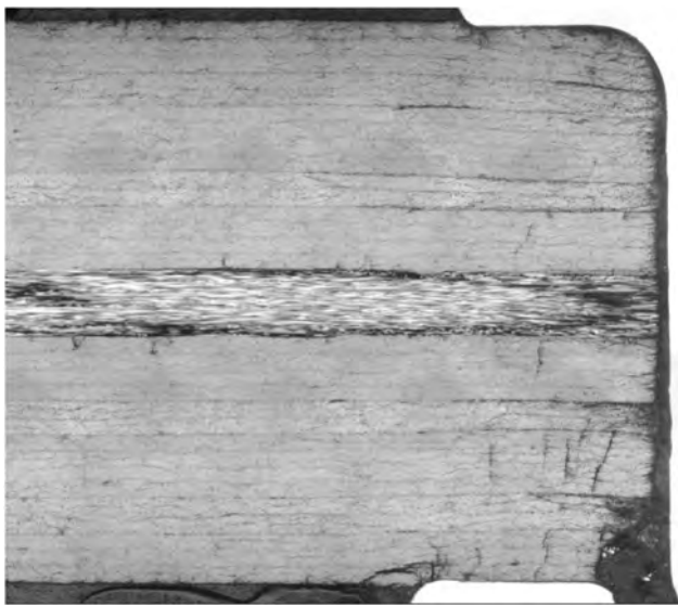
Fig. 23 Detail of the specimen struck with 70 kA, polished perpendicular to the 0 deg fibers in the proximity of the fastener head.
