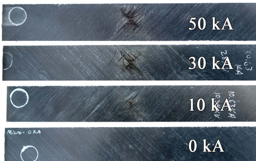
Fig. 8. Typical unnotched specimens, from pristine at the bottom to maximum current at the top.
