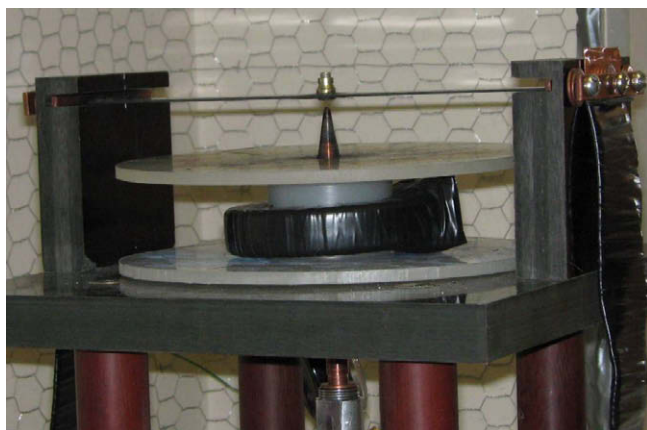
Fig. 4. Detail of the strike and test specimen area of the lightning strike generator.
