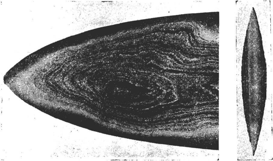
FIG. 26. Macrographic appearance of the point of a Malay kris. Left: (6 diameters) after attack with 5% Nital. Right: Crosswise section (10 diameters). The typical superficial stratification of soft iron is visible (see 500-diameter micrograph below, left), and the central part of hard iron (see 500-diameter micrograph below, right). This latter exhibits grains of ferrite and of martensite together with nodes of troostite, indicators of a rapidhardening thermic treatment.
