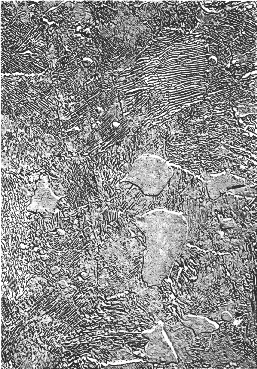
FIG. 12. Electronic micrograph (6,000 diameters) of the Damascus steel from blade No. 1 (see Figures 8 and 10) in the neighborhood of the back. Islands of primary cementite on a field of little-transformed lamellar pearlite (A C copy, shaded with Cr).
