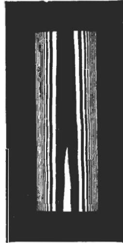
FIGS. 43-44. Cross and longitudinal section of the experimental extruded bar used for the investigation on the manufacturing technique of the «Kirk Narduban». The different layers are clearly shown by the caustic soda etch, which darkens the ones formed with an Al-4% Cu alloy.
