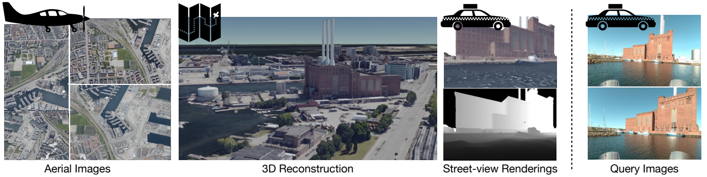
Fig. 4: Street-level-to-aerial localization pipeline. We generate a dense 3D reconstruction from the aerial images. From this reconstruction we render a database of photo-realistic images for real-image-to-render retrieval from street-view queries.
