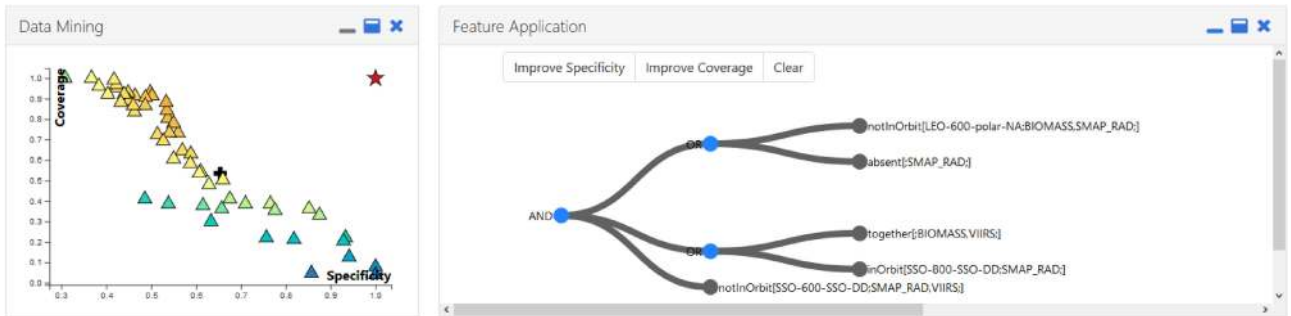
Fig. 4. iFEED Feature space plot and a logical tree representing a feature.
