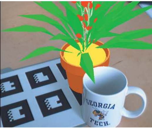
Figure 5: A screenshot of a running DART program. The “program” for this example is shown in Figure 4. There are two objects, the virtual flowerpot, and a “physical” cylinder that is aligned with the cup (hard-coded relative to the fiducial in this example) and used to cause the cup to interact correctly with the flowerpot.
