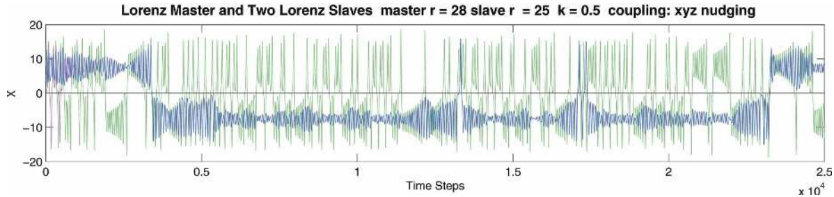
FIG. 5. Two identical slave systems ( r = 25 ) in pink and blue started from different initial conditions coupled to the same master ( r = 28 ) in green. The slaves are coupled to the master through xyz nudging with coupling strength k = 0.5 for which identical synchronization does not occur. The two slaves do not converge with the master but synchronize with each other, which indicates generalized synchronization has been achieved.
