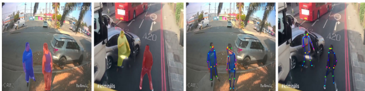
Figure 1: From left to right, the first two images are examples of instance segmentation, the next two examples of pose estimation.
