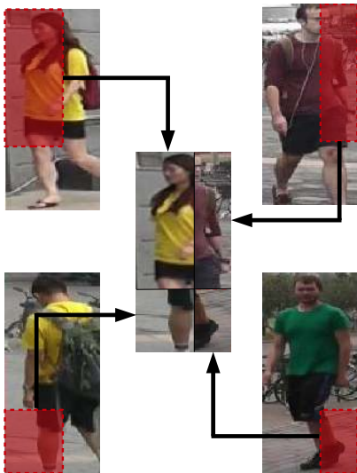
Fig. 10. Conceptual explanation of the proposed fixed image cropping and patching (FICAP) data augmentation. For application of RICAP to person re-identification task, we replaced the random cropping with fixed cropping because of the feature vector matching for image-to-image retrieval.
