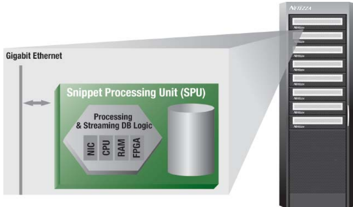
Figure 2. Snippet Processing Units are connected by Gigabit Ethernet to both the host server and to the other SPUs.
